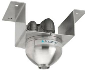
Environmentally friendly AquaMist® SONIC uses readily available water and nitrogen as extinguishing material. Two supersonic atomizers create 1.5 trillion superfine water droplets per second and propel them at high velocity to provide non-toxic fire suppression protection. This system also provides automatic detection and actuation and/or remote manual actuation.
