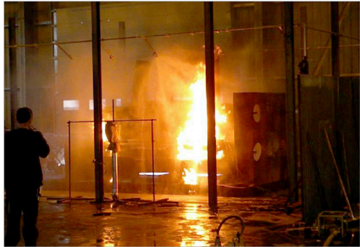
Figure 4 – Burning Leak Tests (the green arrows indicate the two diesel injection points)
